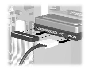
disconnecting the hard disk drive cables
